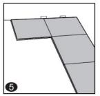
5. **Second row, first tile:** Click the side with the tongue of the tile into the previous row and place an installation wedge under the board (respect the 1/8" / 3 mm expansion gap next to the wall).
