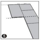
5. **Second row, first tile:** Before starting the second row, mark the center of the second tile in the first row and draw a chalk line / place a string at a 90° angle to the first row following the central line to the opposite wall. Click the side with the tongue of the tile into the previous row and place an installation wedge under the board (respect the 1/8" / 3 mm expansion gap next to the wall).
