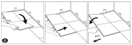
6. **Second row, second tile:** Place the tongue of the second tile at an angle against the grove side of the previously installed tile and fold down. Slide down tongue side of the board into the locking groove of the adjacent tile in the previous row. When the whole row is complete, remove the wedges and fold the row down.
