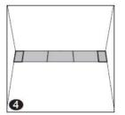
4. **First row, last tile:** At the end of the first row, leave a gap of 1/8"/3 mm to the wall. The last tile should be the same length and width as the first tile.
