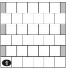
1. **IMPORTANT:** Measure the area to be installed, perimeter rows of opposing walls should be the same width. Adjust the width and the length of the first tile to be installed accordingly.
