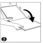
3. **First row, second tile:** Insert the end section of the next tile at an angle. Make sure both tiles are perfectly aligned.
