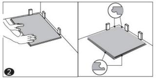
2. **First row, first tile:** After adjusting the measurements of the first tile as described above, begin laying at the left-hand corner of the longest wall and proceed from the wall with the tongue sides facing walls and the grooves facing outward (groove sides are marked with arrows on the back of each tile), away from the walls. Use spacers between the wall and the tile to create 1/8" / 3 mm expansion gap and to keep a straight line parallel to the abutting wall.
