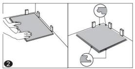
2. **First row, first tile:** After adjusting the measurements of the first tile as described above, begin laying at the left-hand corner of the longest wall and proceed from the wall with the tongue sides facing walls and the grooves facing outward (groove sides are marked with arrows on the back of each tile), away from the walls. Use spacers between the wall and the tile to create 1/8" / 3 mm expansion gap and to keep a straight line parallel to the abutting wall.
