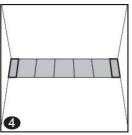
4. **First row, last tile:** At the end of the first row, leave a gap of 1/8"/3 mm to the wall. The last tile should be the same length and width as the first tile.
