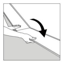
3. **Second plank, first row:** Insert the end section of the next plank at an angle. Make sure both planks are perfectly aligned.
