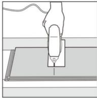
5. If cutting with a jigsaw, the floor surface should be turned down. Otherwise always cut with the floorboard facing up.
