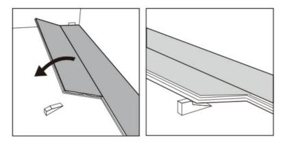
7. Click the long side of the plank into the previous row and place an installation wedge under the board.
