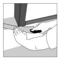
13. **Door molding and skirting:** Lay a board (with the decorative side down) next to the door molding and saw as shown in the figure. Then slide the floorboard under the molding.
