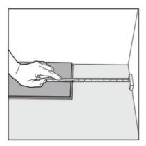
4. At the end of the first row, leave a gap of 1/8" / 3 mm to the wall to avoid any damage while installing your floor, and measure the length of the last plank to fit.
