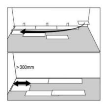
6. Start the second row with a cut off plank. Always ensure that the end joints are staggered at least 8" / 20 cm, both when in the same row as when from one row to the next one. The first plank of the row should be at least 12" / 30 cm in length.
