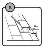
Last Row Use a board to mark the width of the board to be cut. The last row should be at least 50mm wide. The spacers can then be removed. Note: Use a pull bar to ensure last row is in place.
