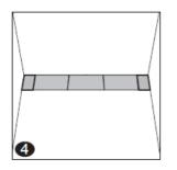
5. **Second row, first tile:** Before starting the second row, mark the center of the second tile in the first row and draw a chalk line / place a string at a 90° angle to the first row following the central line to the opposite wall. Click the side with the tongue of the tile into the previous row and place an installation wedge under the board (respect the min. 3 mm expansion gap next to the wall).
