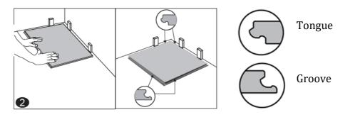
3. **First row, second tile:** Insert the end tongue on the short side of the second tile into the end groove of the first one and rotate downward to assemble. Make sure both tiles are perfectly aligned.
