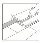
9. **Holes for pipes:** Measure the diameter of the pipe and drill a hole that is 6 mm larger. Saw off a piece as shown in the figure and lay the board in place on the floor. Then lay the sawed-off piece in place.
