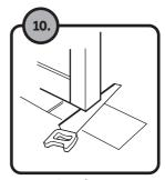
**Door frames** Lay a board (with the decorative side down) next to the door molding and saw as shown. Slide the tile under the moulding.
