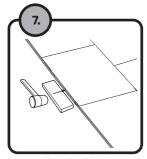
**Tapping Block** (Off-cut of flooring can be used) After the installation of each row. use a mallet & tapping block to tighten the joints.
