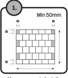
Measure area to install Perimeter rows should be same width. Adjust as required.
