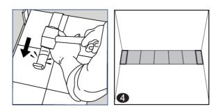
5. **Second row, first tile:** Click the side with the tongue of the tile into the previous row and place an installation wedge under the board (respect the min. 3 mm expansion gap next to the wall).
