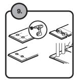
**Holes for pipes** Measure the diameter of the pipe and drill a hole that is 6mm larger. Saw the board removing the piece, lay the board, then re-fit the sawn piece.
